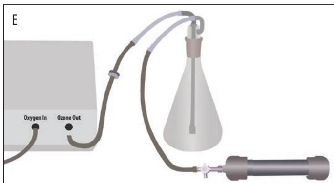
E: Connect the other end of tubing (M) to the base of the ozone destruct system (H).
