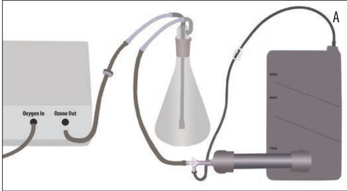
A: When you are ready to fill your insufflation bag, attach the bag (G) to the side port of the ozone destruct system.
