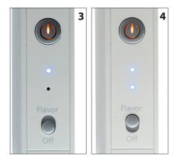
You have successfully used the PHIB device. To power off the unit press the power button quickly three times.
